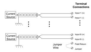
An external source must be provided to power input transceivers.
